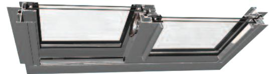
The 8200 Horizontal Sliding Window offers that rare combination of smooth operation, durability, and toughness. It has a 4-1/2" (114 mm) deep frame designed to match typical building conditions, including our entrances and storefronts. An efficient thermally insulated frame accepts 1" (25 mm) glazing. Available in an array of architectural coatings and anodized finishes.
